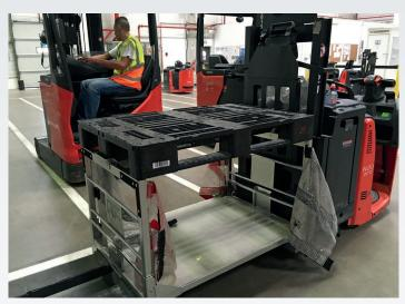
Craemer pallets are positioned on metal collars before being routed through the aisles for order picking.
